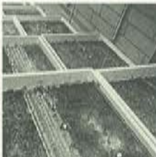
A simulated river flow is used for laboratory studies of how, and how fast, microorganisms degrade chemicals in running water.
