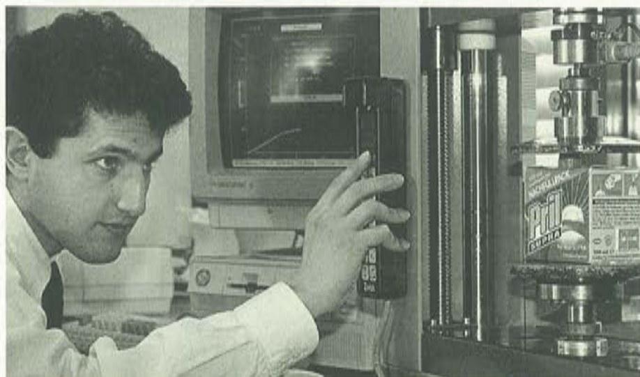
The refill packs for the manual dishwashing agents are also tested, in this case a compression test.
